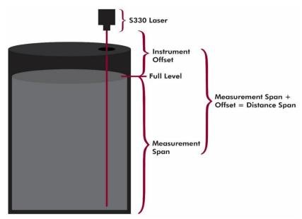
Figure 7: Vessel 4-20 Setup
