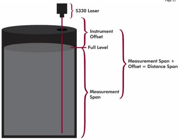
Figure 5: Vessel 4-20 Setup
