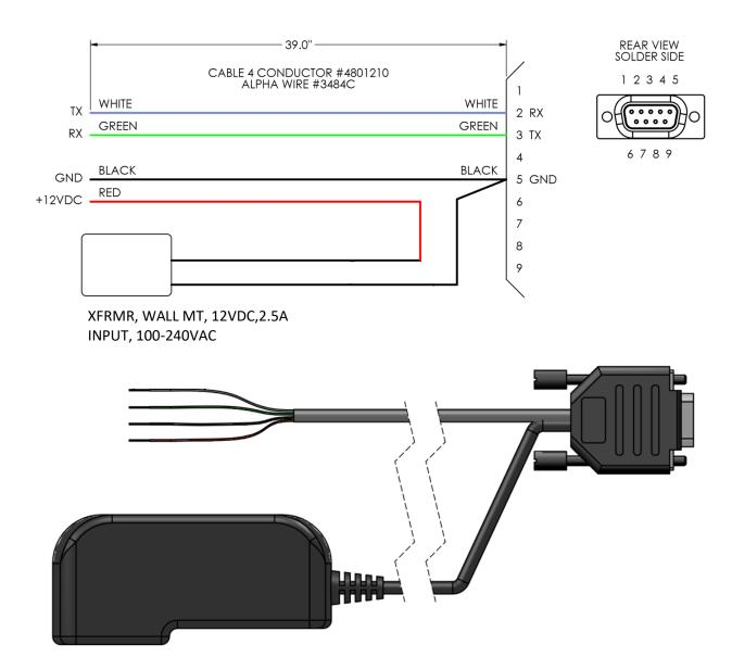
Drawing 4: External Cable Rugged Enclosure
