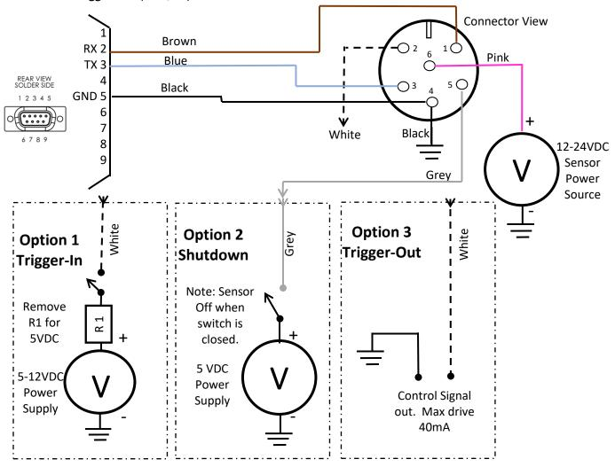
Drawing 7: S300 / S310 I/O Trigger Cable
