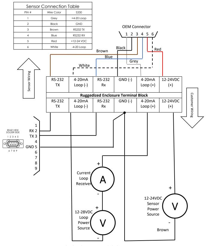
Drawing 6: S330 4-20 Ruggedized Enclosure Terminal Block
