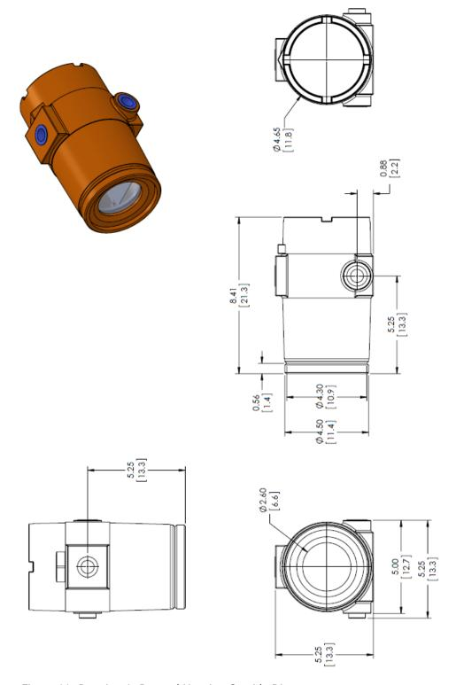
Figure 11: Drawing 1: Rugged Housing Outside Dim.
