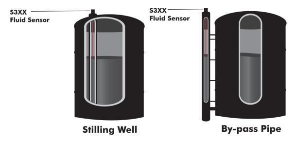
Figure 6: Tank and Vessel Liquid
